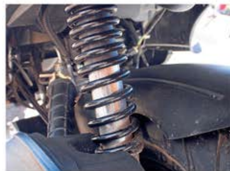
Single rear shock is preload adjustable
